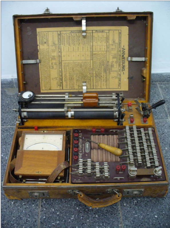
Fig. 5: Portable case with relay testing equipment, manufactured by V&H around 1925
